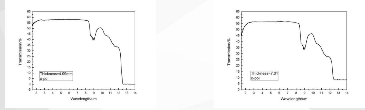
Measured transmission curve of ZnGeP2 crystals
