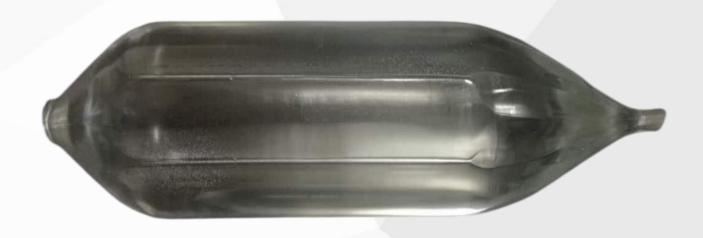
Undoped YAG Crystal or Pure yttrium aluminium garnet provides an interesting alternative to sapphire for UV optics, IR optics and refractometry
