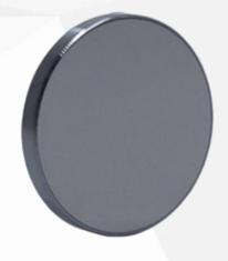
. To avoid this, Silicon can be prepared by a Float-Zone (FZ) process. Optical Silicon is generally lightly doped ( 5 to 40 ohm cm) for best transmission above 10 microns. Silicon has a further pass band 30 to 100 microns which is effective only in very high resistivity uncompensated material. Doping is usually Boron (p-type) and Phosphorus (n-type)
