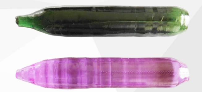
By doping with chromium, the energy absorption capacity of the laser is enhanced and ultra short pulses are emitted. Typical applications of this laser include production of nanopowders and as a pumping source for other lasers.
