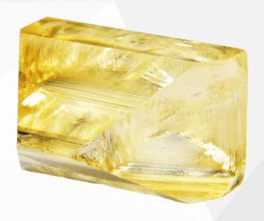
KTA is often used as an OPO / OPA gain medium for emission in the  $3\mu m$  range as well as an OPO crystal for eye-safe emission at high average power.
