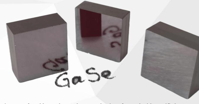
GaSe is very soft and layered crystal. For production of crystal with specified thickness we take thicker starting blank ,For example, 1-2 mm thick and then begin to remove layer by layer trying to approach to ordered thickness while keeping good surface smoothness and flatness. However, for thicknesses about 0.2-0.3 mm or less GaSe plate easily bends and we obtain curved surface instead of flat one.
