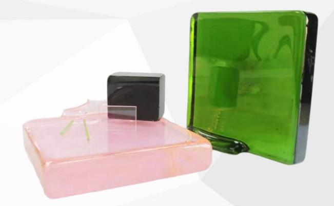
Erbium Glass doped with Er 3+ and Yb 3+ and suited to applications involving high repetition rates (1 - 6 Hz) and being pumped with 1535 nm laser diodes. This glass is available with high levels of Erbium (up to 1.7%).
