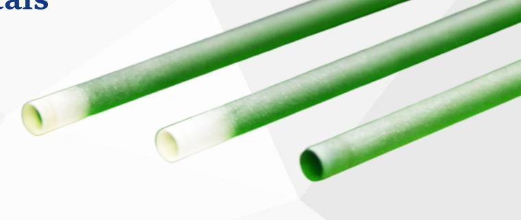
Cr, Tm, Ho: YAG is high efficient laser crystal pumped by Xenon lamp or diode with wavelength of 2.1 $\mu$ m. the pump source main originates from the flashlamp energy absorbed by Cr3+, Ho3+ is working ion and Tm3+ acts as intermediary to transfer energy. 2.1  $\mu$ m laser wave can be absorbed by water very well, transmits atmosphere easily and is safe to eye.
