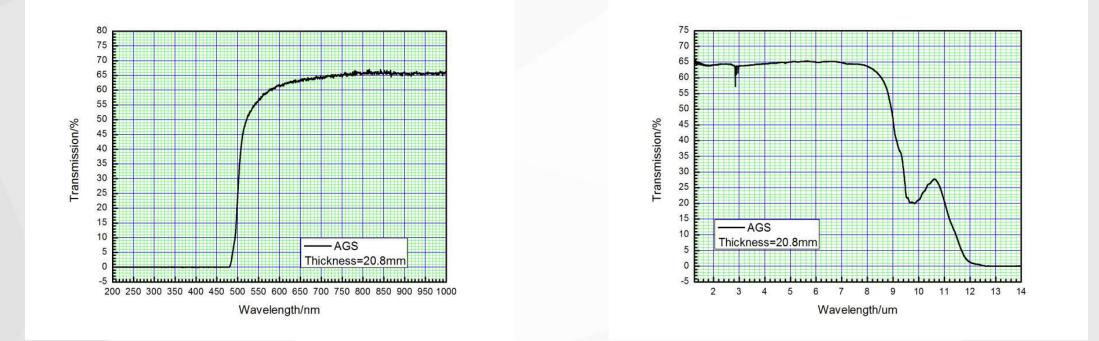
Measured transmission curve of AgGaS2 crystals
