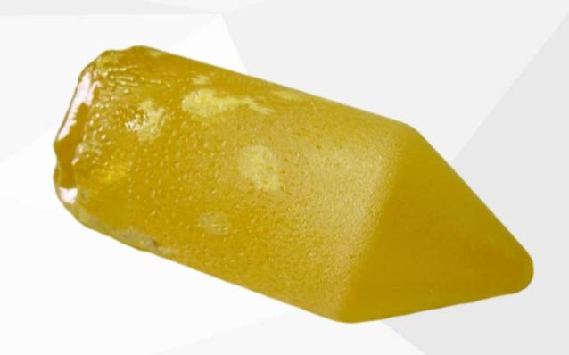
Due to its higher damage thresholdand greater variety of phase-matching schemes AgGaGeS4 could become an alternative to the widely spread now AgGaS2 in high power and specifific applications.
