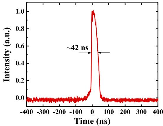
Fig. 3. Pulse width measurement of the idler light at 6.45  $\mu\text{m}$ .
