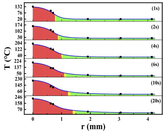
Fig. 5. Temperature distribution on the ablated tissue surface with respect to the center point of the irradiation position for different irradiation durations. The black squares are the measured data. The solid curves are the simulated results. The left shaded zone is where the temperature  $T$  exceeds 60°C. The middle shaded zone is where  $55^\circ\text{C} \leq T < 60^\circ\text{C}$ , and the right shaded zone is where  $T < 55^\circ\text{C}$ .
