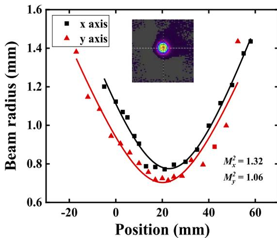
Fig. 4. Beam quality factor measurement of the 6.45  $\mu\text{m}$  idler. Inset: 2D beam intensity profile.
