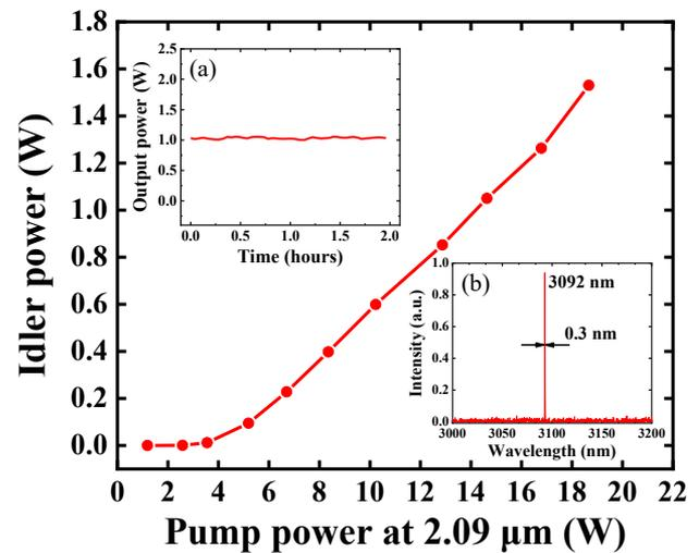
**Fig. 2.** Output power at 6.45  $\mu\text{m}$  versus pump power at 2.09  $\mu\text{m}$ . Insets: (a) signal spectrum of the ZGP-OPO; (b) measured power stability of the idler at 6.45  $\mu\text{m}$  over 2 h.
