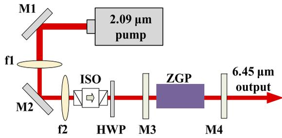
**Fig. 1.** Experimental arrangement of the 6.45  $\mu\text{m}$  ZGP-OPO system.
